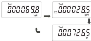
Switching between information displays for three-phase meters [1]
